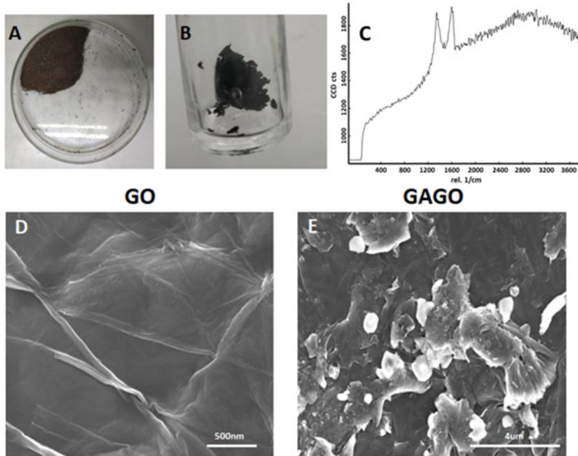
Figure 1. (A) GO flakes synthesized by a modified Hummer’s method (B) Freshly prepared GA loaded GO (GAGO). (C) Raman spectra of GO obtained at 532 nm. FESEM images of (D) GO and (E) GAGO at 100x magnification. Scale bar represents 500 nm for GO and 4  $\mu\text{m}$  for GAGO.
